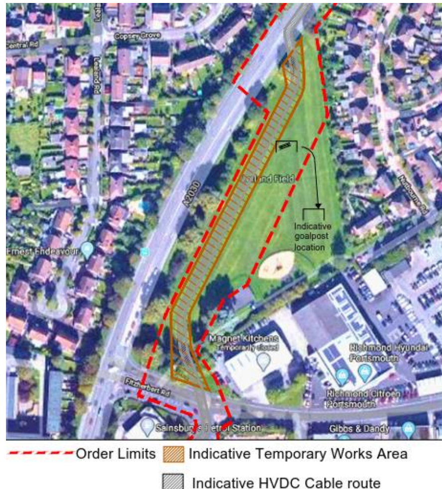
Plate 9 - Zetland Field, indicative construction layout
